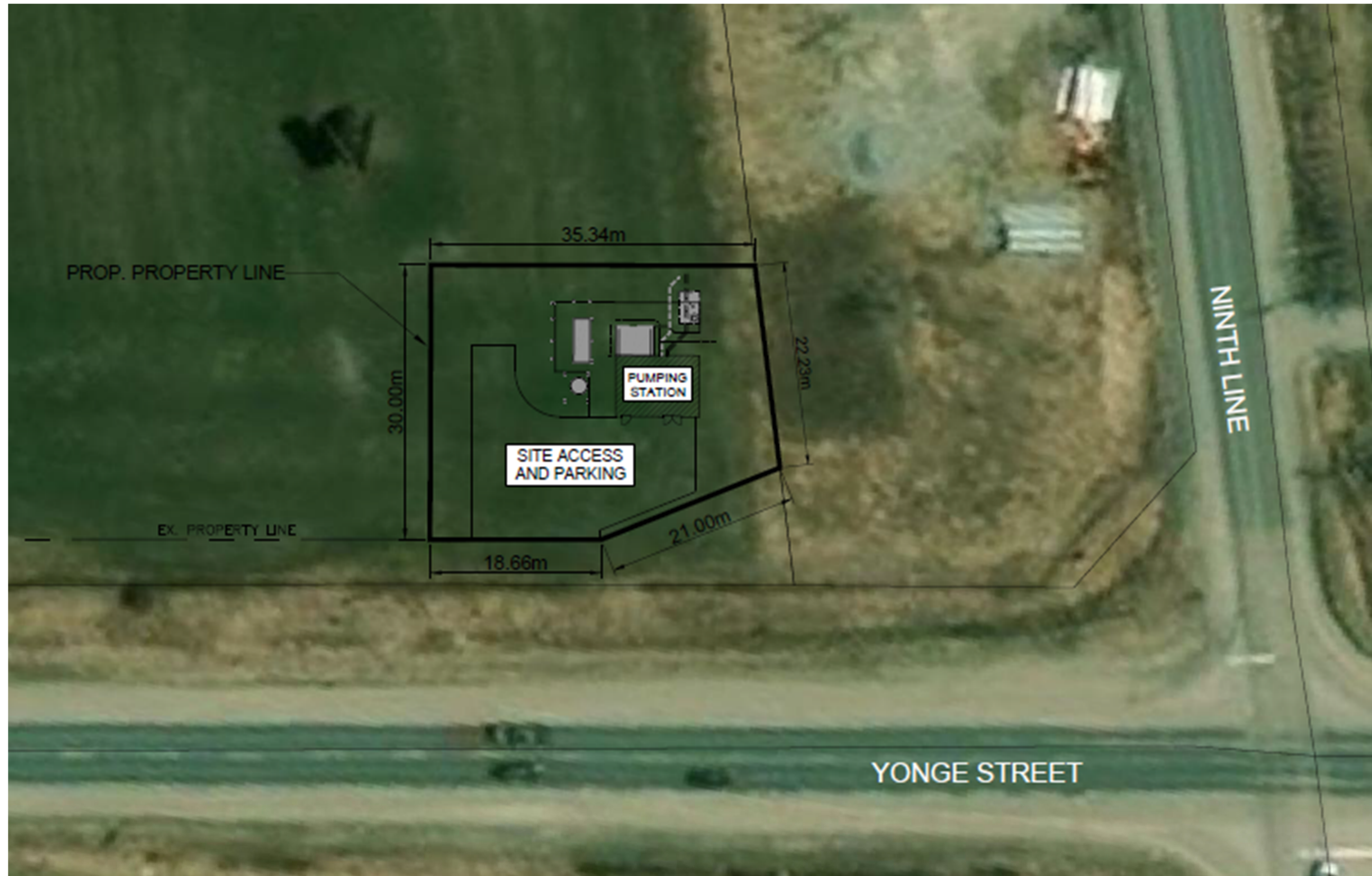
Figure 12 – Preliminary Layout of the SPS
